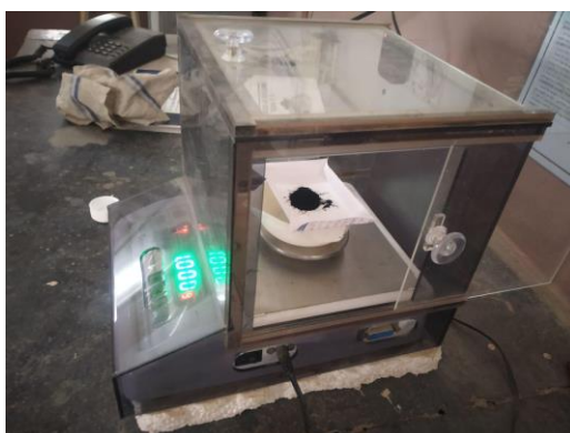
Fig 2. Measurement of Graphene powder using digital weighing
